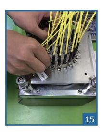
13.Install The Boot with The Connector until it stays well and not loose.
